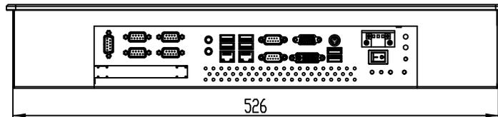
CUT OUT DIMENSION(528x352mm) UNIT:mm
